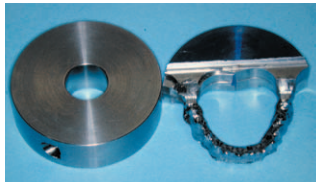
Figure 2 Left, a solid block of titanium. Right, a completed framework before separation from the block.
