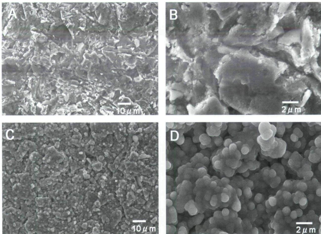
**Figure 1** Scanning electron microscopy images showing the surface structures of the control disk (A and B;  $\times 1000$  original magnification) and the anatase  $\text{TiO}_2$ -covered disk (C and D;  $\times 4000$  original magnification).
