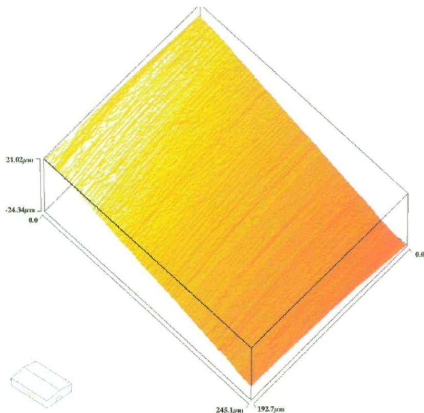
**Figure 1** A turned flank. Marks produced by the cutting tool during turning are clearly visible. These marks give the surface the dominating direction of the irregularities perpendicular to the long axis of the implant.
