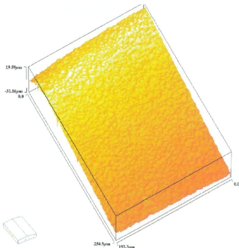
Figure 2 A turned and blasted flank. The blasting procedure has removed the turning marks, and the surface no longer has a dominating direction.
