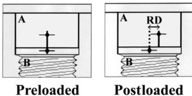
**Figure 2** Schematic diagram showing preloaded and postloaded conditions an abutment (A) and implant (B) with a crossing hand-drawn vertical line and two horizontal lines. RD = rotational displacement.
