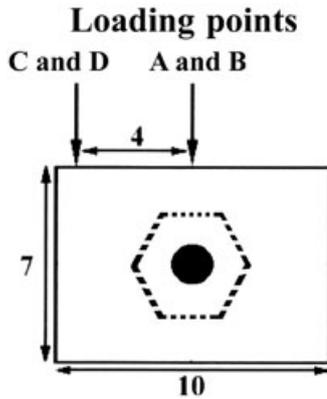
**Figure 1** Schematic diagram showing the loading conditions for test groups from the top or occlusal view. The dotted hexagon represents the implant or abutment hexagon, and the central black circle indicates the screw head access hole for tightening.
