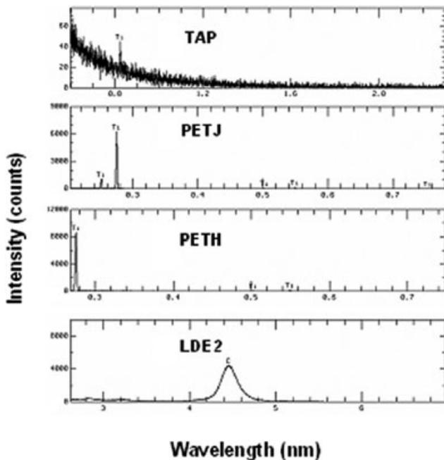
**Figure 5** Electron probe micro-analyzer data of the experimental implant. The analyzing crystals for EPMA qualitative analysis were thallium acid phthalate (TAP), pentaerythritol(J) (PETJ), pentaerythritol(H) (PETH), and layered dispersion element 2 (LDE2). Titanium (Ti) was detected in addition to carbon (C) from the plastic, and the presence of titanium on the surface was confirmed. Other impurities were not detected.
