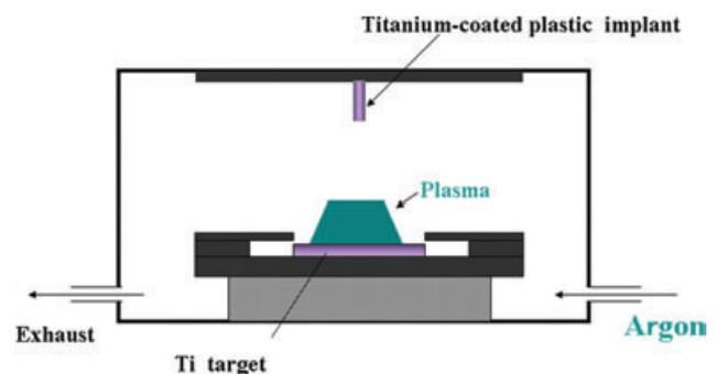
**Figure 1** The schema of the DC magnetron sputtering apparatus. A 99.9% pure titanium target was used. The apparatus was filled with argon. The generated argon plasma and target were used to produce titanium ions, and the plastic implant surface was coated.
