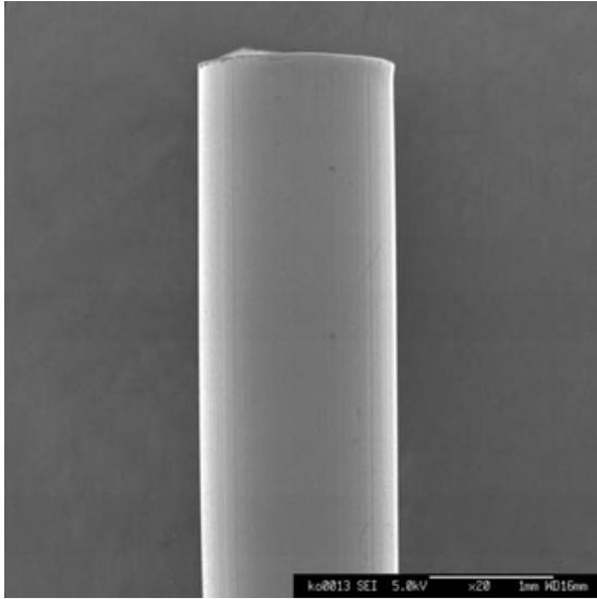
**Figure 4** Scanning electron microscopy image of the experimental implant. The surface was mostly smooth, and the surface morphology of the plastic prior to coating was mostly preserved.
