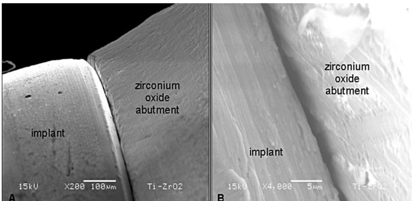
**Figure 4** A and B, Scanning electron microscope photographs of zirconium oxide abutment group before the dynamic loading.
