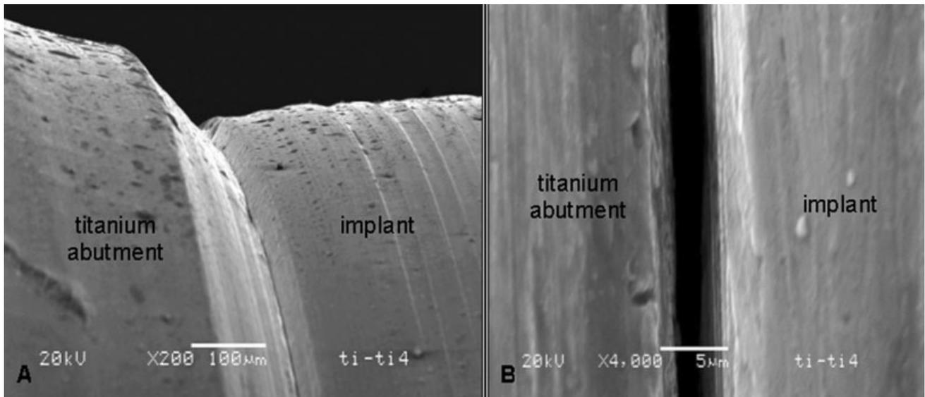
**Figure 5** A and B, Scanning electron microscope photographs of titanium abutment group before the dynamic loading.
