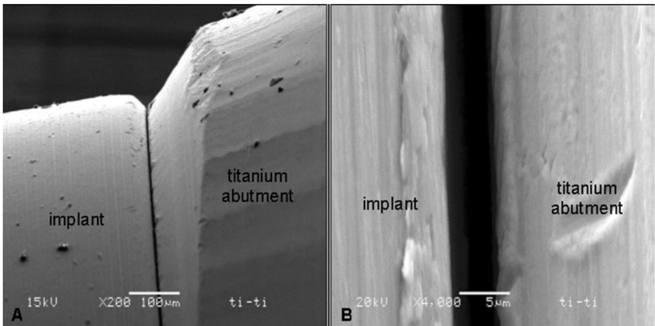
Figure 8 A and B, Scanning electron microscope photographs of titanium abutment group after the dynamic loading.
