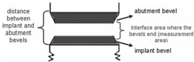
**Figure 1** The diagram of the measurement area between the implant-abutment interface.
