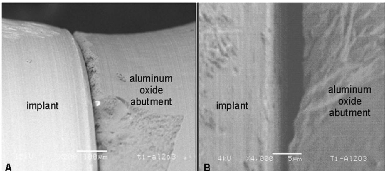
**Figure 6** A and B, Scanning electron microscope photographs of aluminum oxide abutment group after the dynamic loading.
