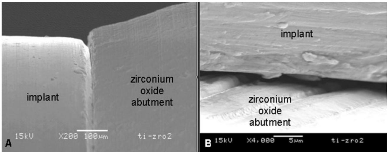
Figure 7 A and B, Scanning electron microscope photographs of zirconium oxide abutment group after the dynamic loading.
