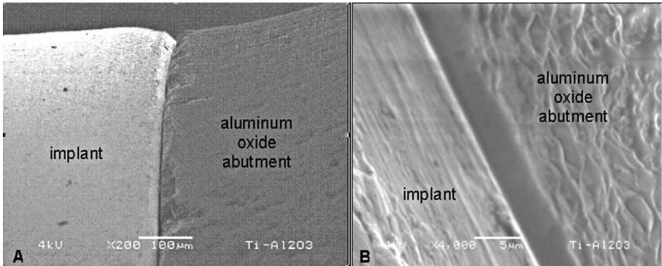
**Figure 3** A and B, Scanning electron microscope photographs of aluminum oxide abutment group before the dynamic loading.
