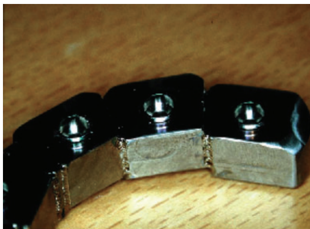
Figure 2 The “third generation” of laser-welded titanium framework (Ti-3) with vertical laser-welding joints.
