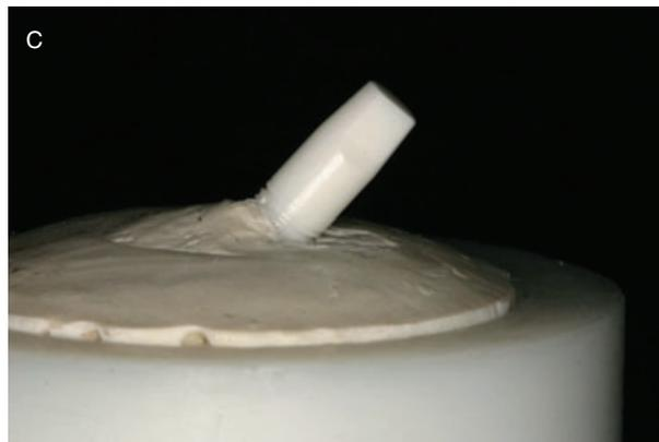
**Figure 1** A, Outline of the study; B, (left) an implant of group D (Y-TZP-A BIO-HIP® implant), (right) chamfer preparation of a ZiUnite® implant (group F); C, a ZiUnite implant embedded in the sample holder (inclination angle of 130°).
