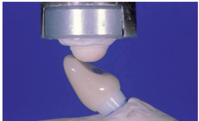
**Figure 2** Implant/crown system subjected to artificial load.
