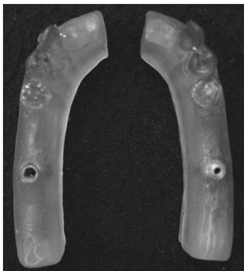
**Figure 2** Photoelastic models: external hexagon (*left*); internal hexagon (*right*).
