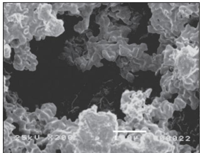
**Figure 2** Scanning electron microscopy showing Ti-foam architecture.
