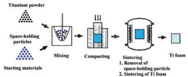
**Figure 1** Schematic illustration of Ti-foam fabrication. Published in Wen et al. (2002).<sup>7</sup>
