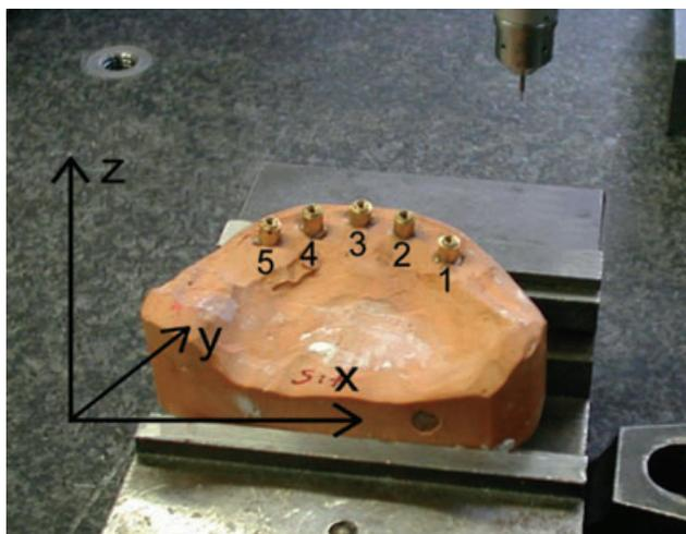
**Figure 3** Coordinate system (x-, y-, and z-axes) and setup of CMM measuring machine for the measurements. Master model with implant replicas numbered from 1 (right) to 5 (left) mounted in the mold.
