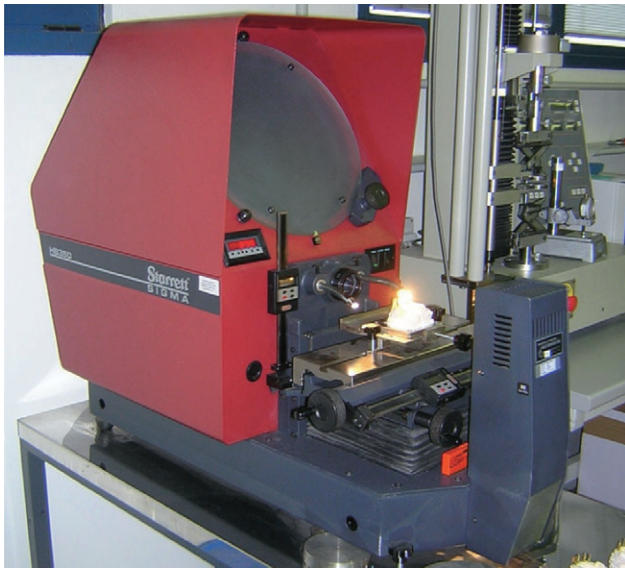
Figure 7 The profile projector used for the measurements.
