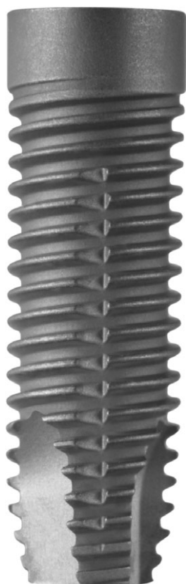
Figure 1 Design of the Neoss™ implant used in the study. The implant has a 1.9-mm high collar and a threaded body with a positive tolerance and vertical flutes. The Bimodal™ surface is achieved by blasting with two different sizes of ceramic particles.
