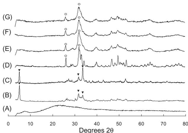
**Figure 4** XRD patterns of (A) collagen, (B) OCP, (C) OCP/collagen, (D) HA, (E) dog bone and OCP/collagen implanted for (F) 3 or (G) 6 months. (▼) OCP reflection. (○) Apatite reflection.
