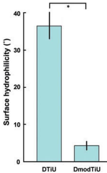
**Figure 1** Water contact angle of DTiU and DmodTiU (\* $p < .05$ ).
