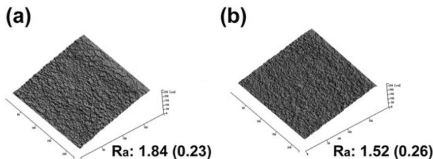
**Figure 2** Laser three-dimensional microscopic images of (A) TiU with an average Ra value of 1.84 (0.23) and (B) modTiU with an average Ra value of 1.52 (0.26). (Ra = average roughness.)
