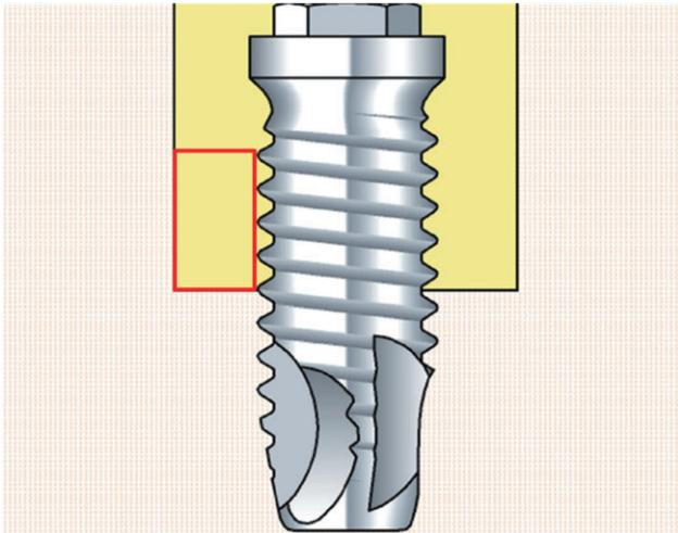
**Figure 2** Schematic drawing of a dental implant installed in a circumferential bone defect (6.3 mm in diameter and 5.0 mm in depth). BAR region is highlighted in red.
