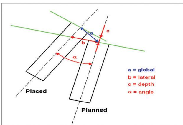
**Figure 3** Three-dimensional evaluation of the virtually planned and the in vivo placed implants.
