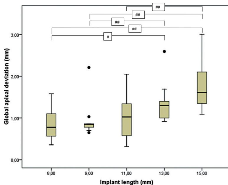
**Figure 5** Box plot showing median, quartile, range, and outliers of global apical deviations (in mm) of 77 implants. The extreme outliers represent initially unstable implants. Bars represent statistically significant differences (Mann-Whitney *U* test; #*p* < .05; ##*p* < .01).
