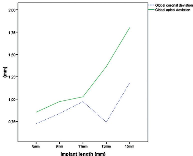
**Figure 6** Mean global coronal and mean global apical deviation related to the different implant lengths used.
