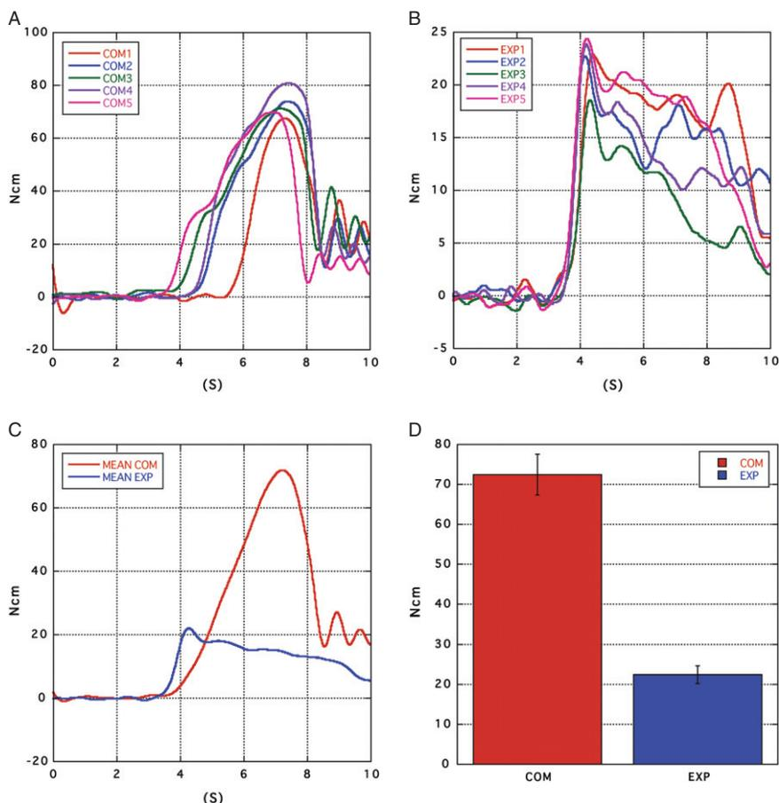
**Figure 2** (A) Removal torque curves for all commercial implants placed in gypsum type 3 ( $n = 5$ ; COM1-COM5). (B) Removal torque curves for all experimental implants placed in gypsum type 3 ( $n = 5$ ; EXP1-EXP5). (C) Removal torque curves (mean values) for the commercial implants and the experimental implants. (D) Graph showing the mean peak values in Ncm and SD for the two groups (COM: 72.50 [5.1]; EXP: 22.40 [2.2]).
