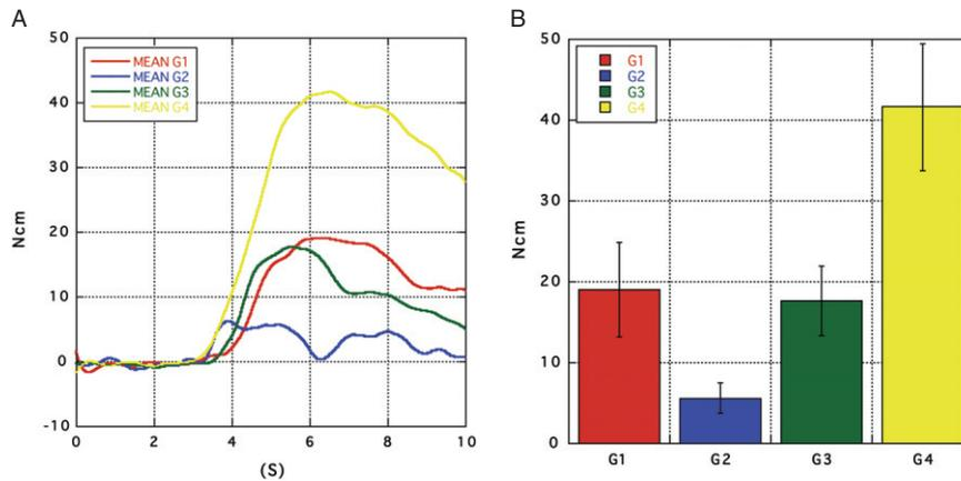
**Figure 1** (A) Removal torque curves (mean values) for implants placed in different gypsums ( $n = 5$ ; G1–G4). (B) Graph showing the mean peak values in Ncm and standard deviation (SD) for all groups (G1: 19.0 [5.9]; G2: 5.6 [1.9]; G3: 17.7 [4.3]; G4: 41.6 [7.8]).
