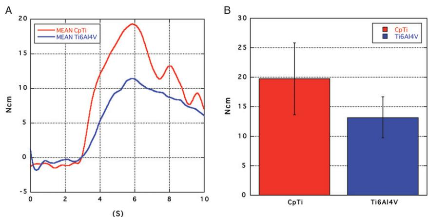
**Figure 3** (A) Removal torque curves (mean values) for the cpTi implants and the Ti6Al4V implants placed in rabbits after 6 weeks ( $n = 4$ ). (B) Similar data presented as graphs with SD. The mean values (Ncm) for cpTi: 19.75 and for the Ti6Al4V: 13.20.
