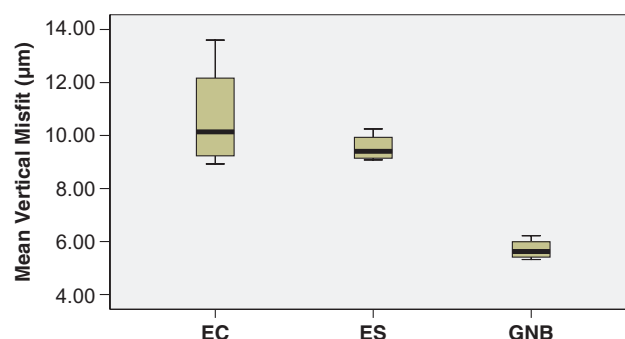
Figure 1 Box plot comparing misfit at implant-abutment interface for each group. EC = Procera abutment associated with implants from Conexão. ES = Procera abutment associated with implants from SIN. GNB = Procera abutment associated with implants from Nobel Biocare.
