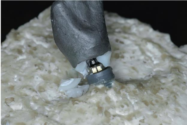
**Figure 3** A representative image of fractured test specimen (group Zr-8). Metal part of the abutment is shown. Zr = zirconia.
