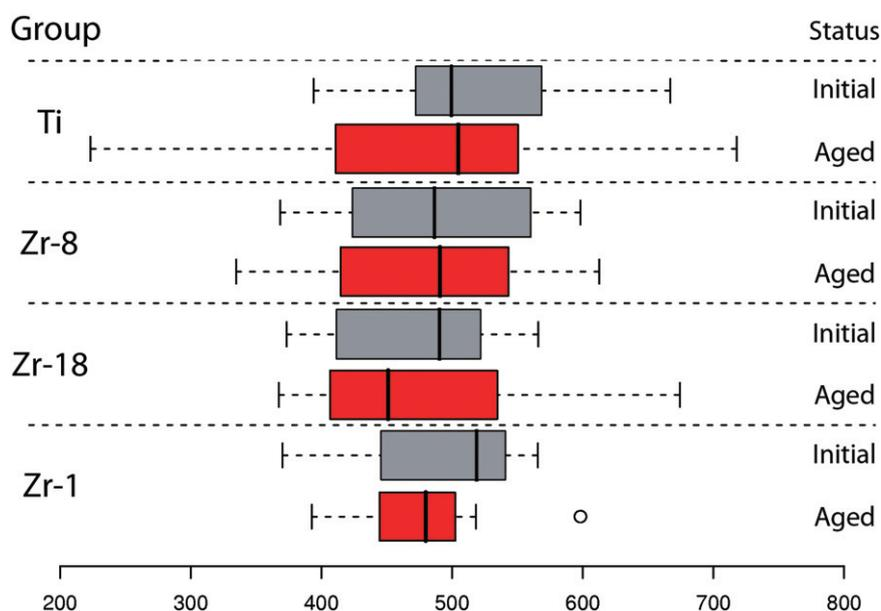
**Figure 4** Box plots of the results after the load-to-fracture test in N before and after the fatigue loading ( $n = 8$ ). Pairwise comparisons did not yield statistical differences between and within groups, before and after artificial aging ( $p > .05$ ). Ti = titanium abutments (control group); Zr-1 = zirconia abutments with a wall thickness of 1 mm; Zr-8 = zirconia abutments with a wall thickness of 0.8 mm; Zr-18 = zirconia abutments with a wall thickness reduced from 1 mm to 0.8 mm.
