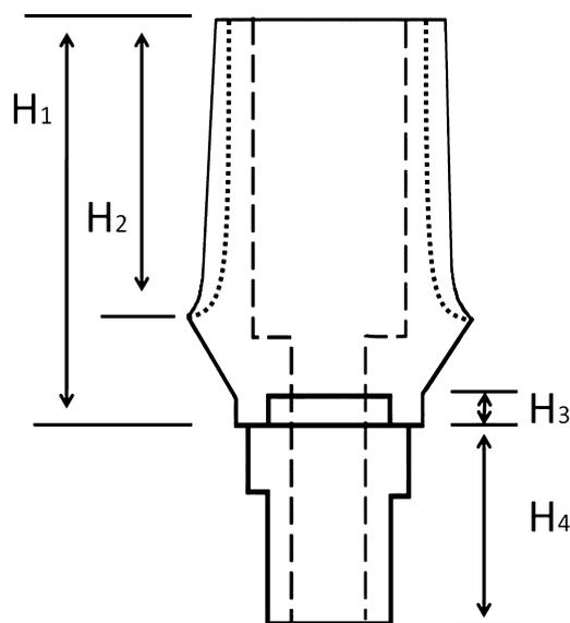
**Figure 1** A schematic drawing of the abutment configuration of different groups (abutment height [H1]: 9.5 mm, clinical height [H2]: 7 mm, height of metal basis [H3]: 1 mm, height of intra-implant portion [H4]: 3.75 mm). Dotted line denotes the reduction of wall thickness from original abutment size in group Zr-18. Zr = zirconia.
