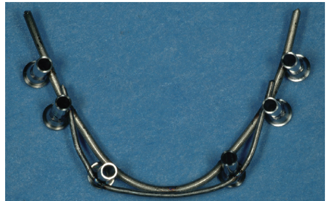
Figure 7 The titanium framework immediately after retrieval.
