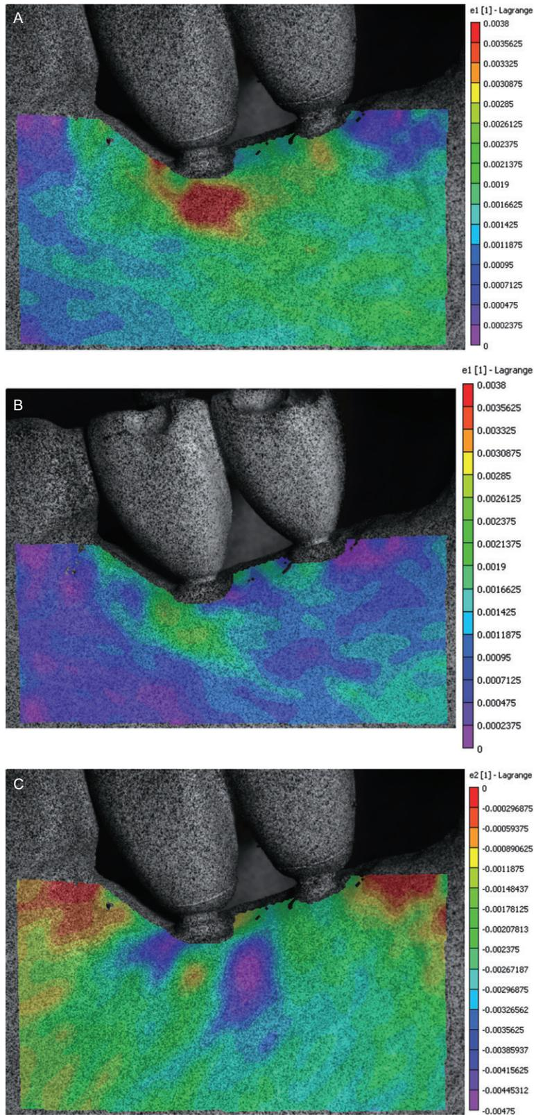
**Figure 5** A, Patterns of strain for oblique loading on splinted prostheses, maximum principal strain for cement-retained. B, Patterns of strain for oblique loading on splinted prostheses, maximum principal strain for screw-retained. C, Patterns of strain for oblique loading on splinted prostheses, minimum principal strain for cement-retained.
