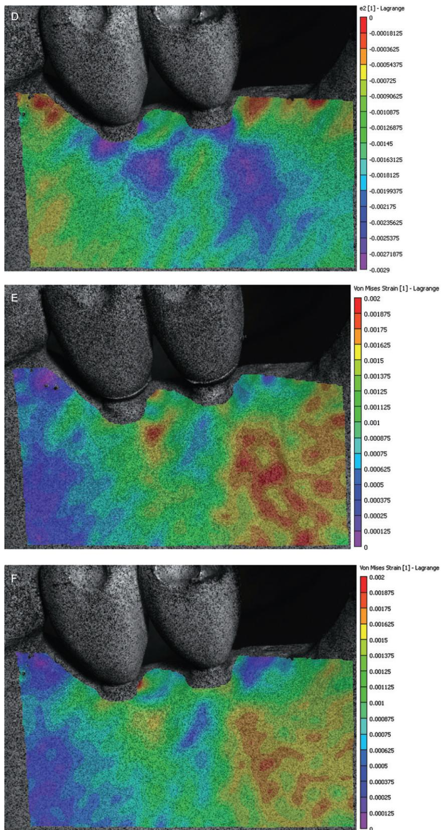
**Figure 3** (continued) *D*, Patterns of strain for vertical loading on splinted prostheses, minimum principal strain for screw-retained. *E*, Patterns of strain for vertical loading on splinted prostheses, von Mises equivalent strain for cement-retained. *F*, Patterns of strain for oblique loading on splinted prostheses, von Mises equivalent strain for screw-retained.
