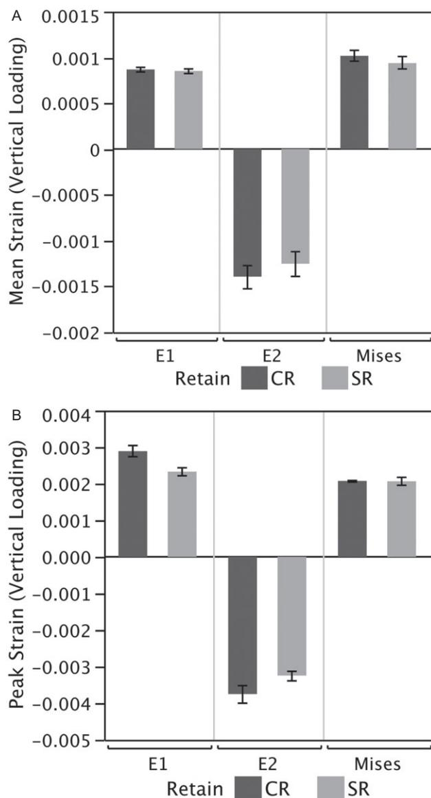
**Figure 4** A, Mean major (E1), minor (E2), and von Mises strains for cement-retained (CR) and screw-retained (SR) splinted crowns with vertical loading. B, Peak strains for cement-retained (CR) and screw-retained (SR) splinted crowns with vertical loading.
