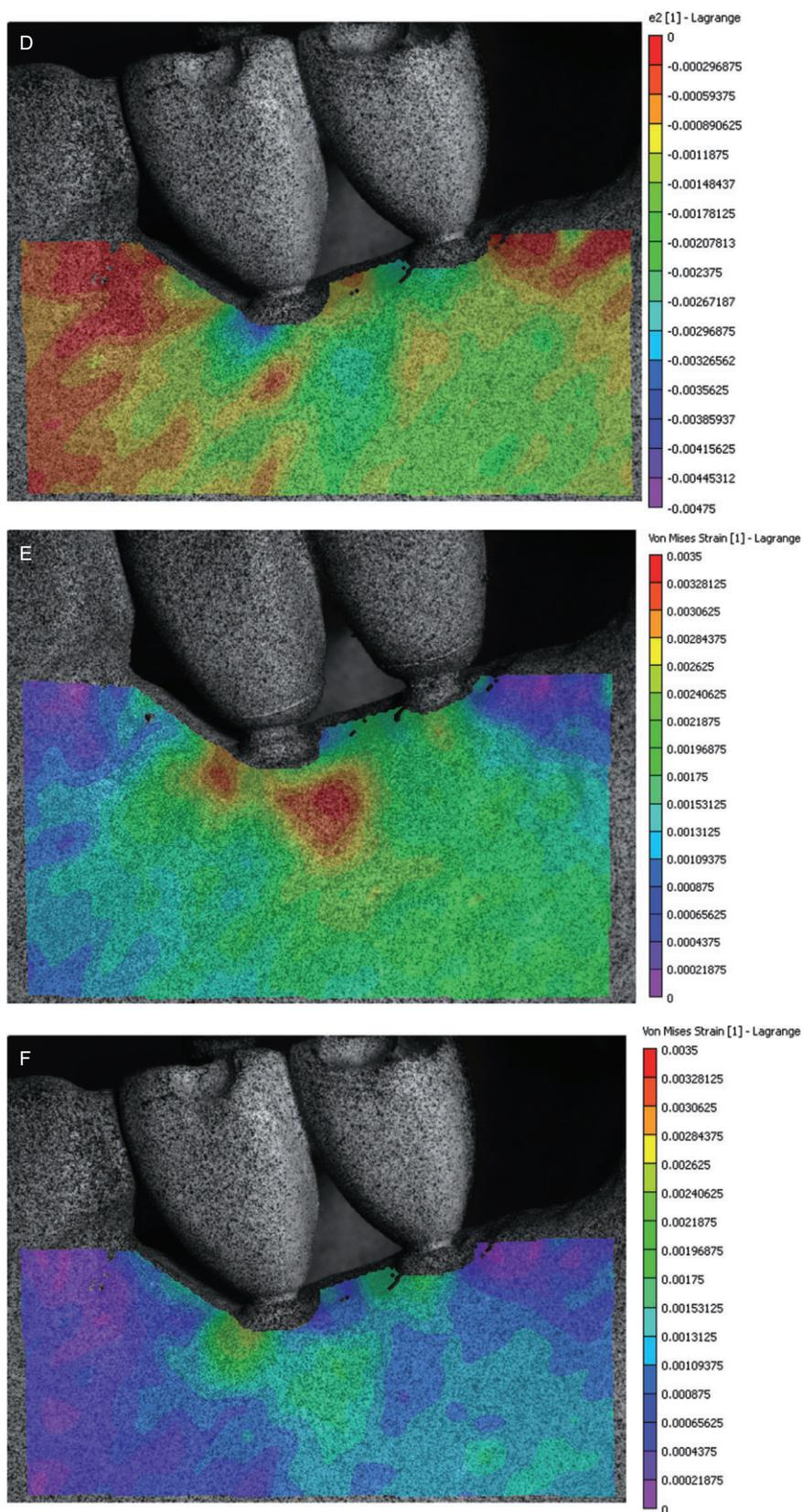
**Figure 5** (continued) *D*, Patterns of strain for oblique loading on splinted prostheses, minimum principal strain for screw-retained. *E*, Patterns of strain for oblique loading on splinted prostheses, von Mises equivalent strain for cement-retained. *F*, Patterns of strain for oblique loading on splinted prostheses, von Mises equivalent strain for screw-retained.
