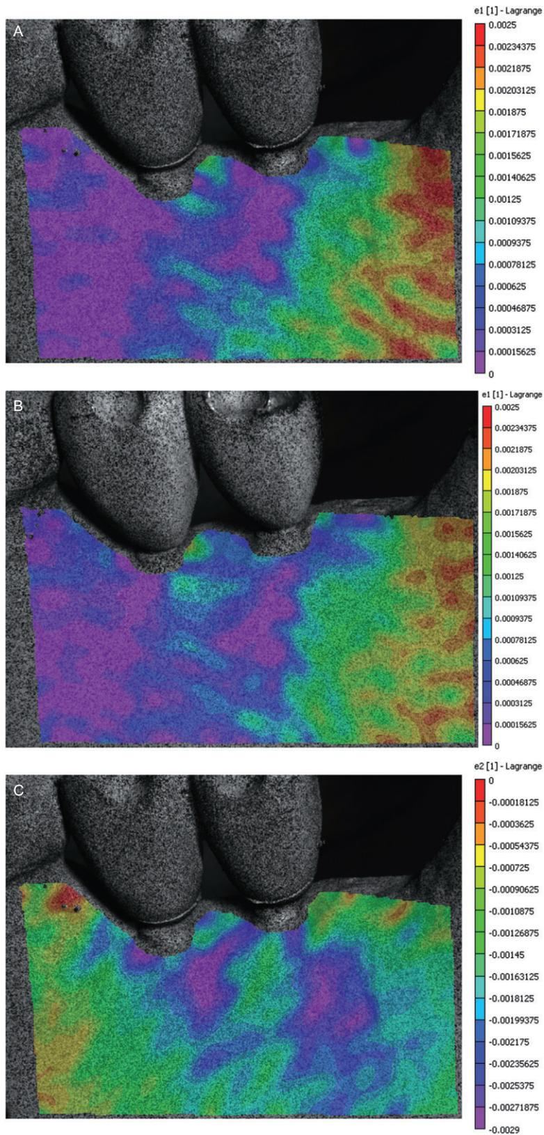
**Figure 3** A, Patterns of strain for vertical loading on splinted prostheses, maximum principal strain for cement-retained. B, Patterns of strain for vertical loading on splinted prostheses, maximum principal strain for screw-retained. C, Patterns of strain for vertical loading on splinted prostheses, minimum principal strain for cement-retained.
