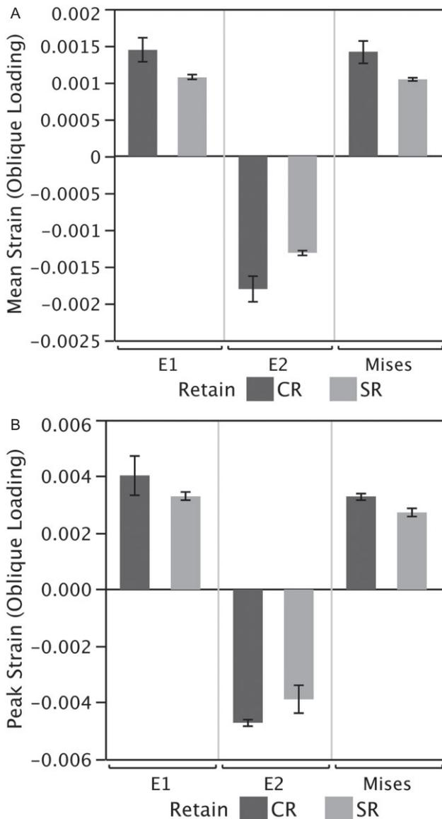
**Figure 6** A, Mean major (E1), minor (E2), and von Mises strains for cement-retained (CR) and screw-retained (SR) splinted crowns with oblique loading. B, Peak strains for cement-retained (CR) and screw-retained (SR) splinted crowns with oblique loading.
