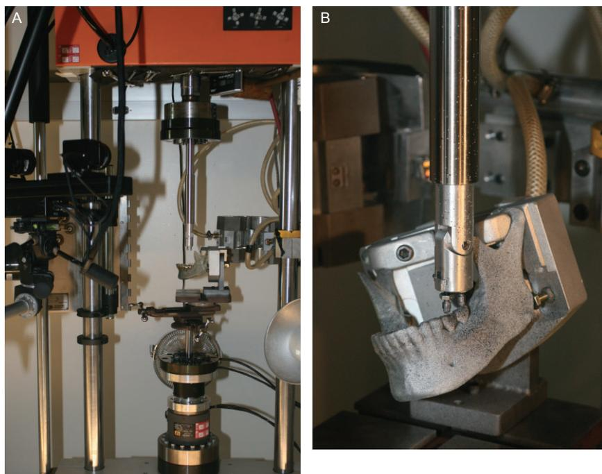
**Figure 2** A, Universal testing machine and dual camera apparatus for vertical loading. B, Oblique loading position.
