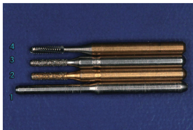
Figure 1 The four dental burs were (Strauss Co., Raanana, Israel) (1) a smooth surface bur; (2) Premium Line diamond D1PR/medium grains; (3) regular diamond D1/medium grains; and (4) carbide FGB 1557.
