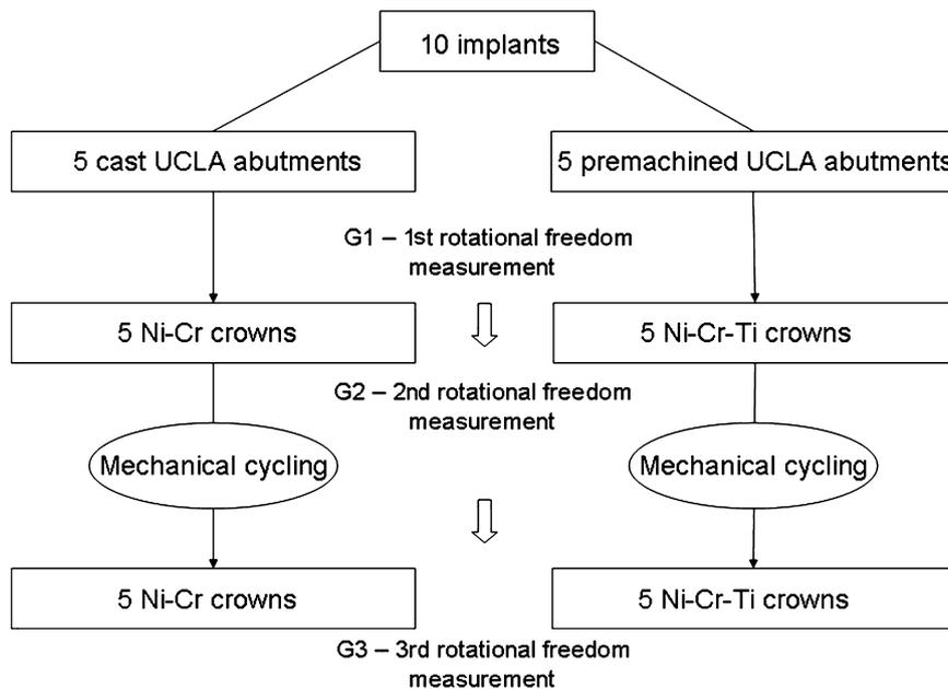
**Figure 2** Schematic representation of the experimental groups. Ni-Cr = nickel-chromium alloy; Ni-Cr-Ti = nickel-chromium-titanium alloy; UCLA = University of California, Los Angeles.
