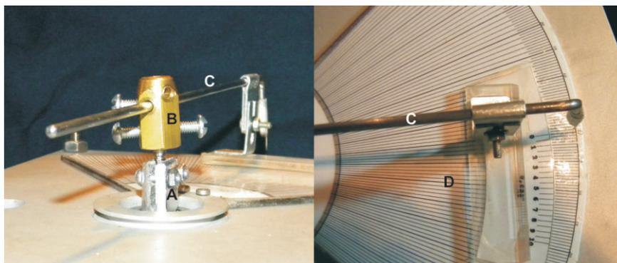
**Figure 1** Experimental device designed to measure rotational freedom angles between the abutment and implant. A and B, Devices for locking the implant (A) and abutment (B). C, Rod to measure rotational freedom. D, Graduated scale with 0.025°.
