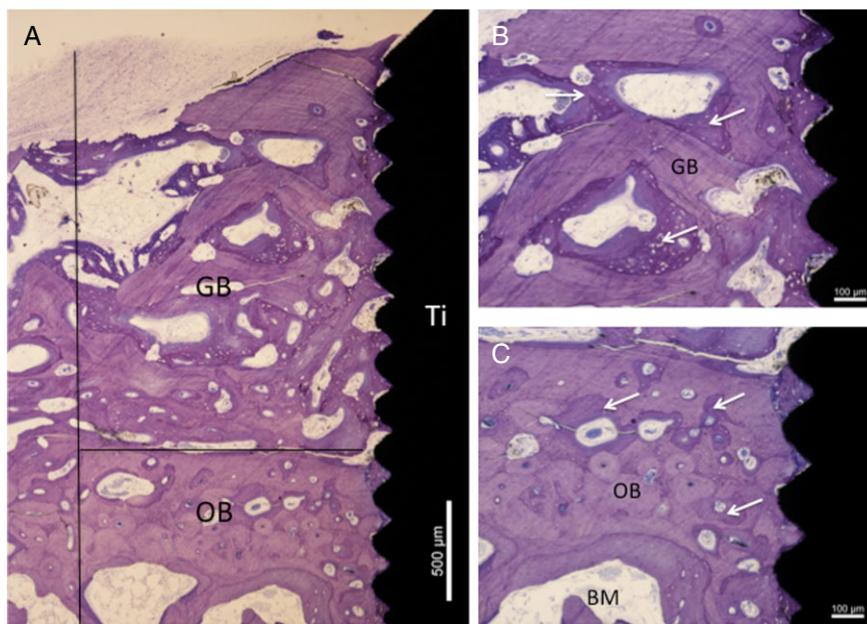
**Figure 1** Light micrographs of a test specimen after 8 weeks of healing. *A*, Overview. The implant (Ti) seems to be well integrated in both grafted (GB) and original bone (OB). Bar = 500  $\mu$ m. *B*, Close up of grafted area showing an admixture of GB and newly formed immature bone (arrows). Bar = 100  $\mu$ m. *C*, Close up of the original cortical bone showing new secondary osteons (arrows). Bar = 100  $\mu$ m.
