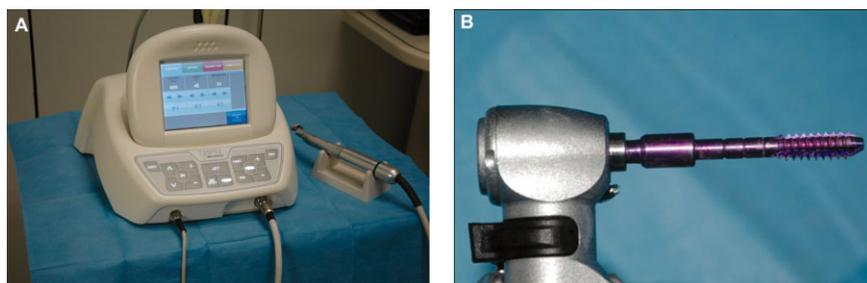
**Figure 1** A, The computerized implant motor able to assess the value of bone cutting resistance and obtain an Intraoperative Density Index. B, Bone density reading drill mounted handpiece.
