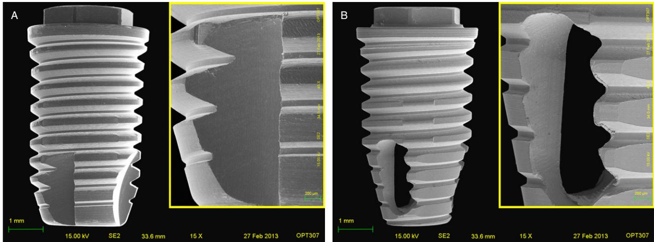
**Figure 1** Scanning electron microscopy (SEM) micrograph of the control (A) and test (B) implants. The difference between the groups is limited to the apical third. Test implants reveal an apical hollow chamber with eccentric cutting edges. Coronal and middle thirds of control and test implants are identical.
