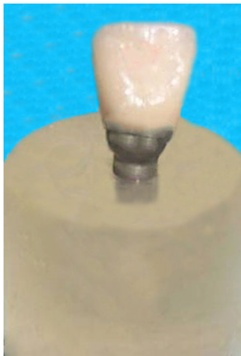
Figure 2 Ceramometal crown cemented over titanium abutments embedded in clear acrylic resin.
