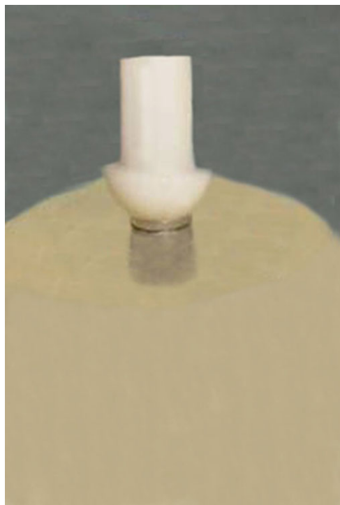
Figure 1 Zirconia abutment embedded in clear acrylic resin.
