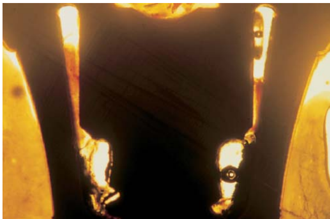
Fig. 5 Photomicrograph of implant's coronal portion with closure screw, demonstrating internal Morse taper and external flaring of the neck ( \times 25 )
