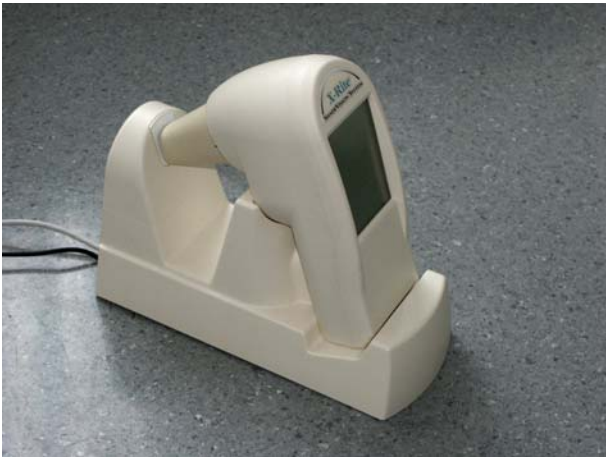
Fig. 2 X-Rite ShadeVision handset (colorimeter) with universal serial bus (USB) docking station
