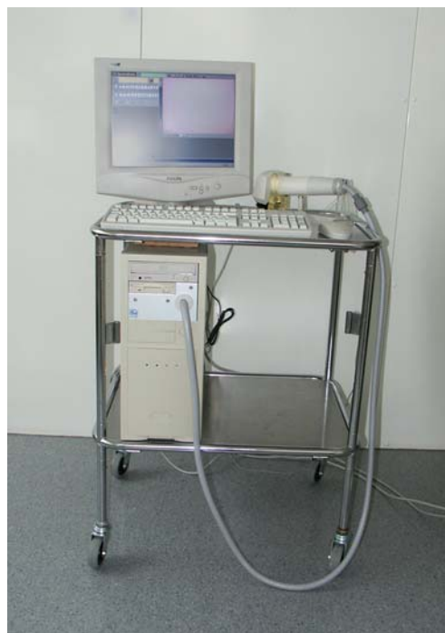
Fig. 1 MHT SpectroShade unit with Spectrophotometer integrated into the computer casing
