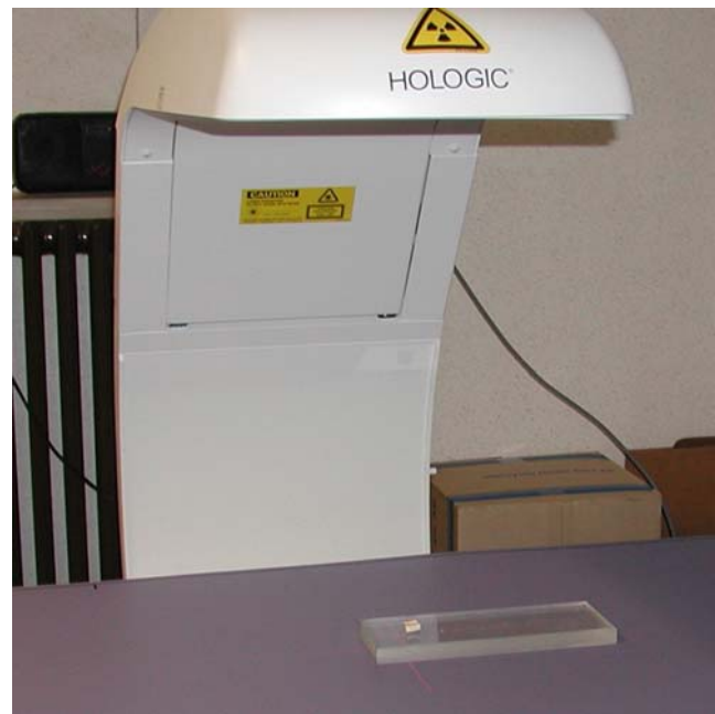
Fig. 1 DXA scanner with bone sample on plexi
