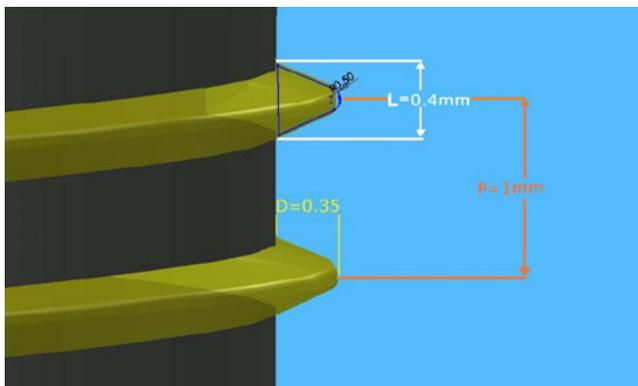
**Fig. 1** Schematic illustration of thread profile properties used in study. Threads pitch ( $P$ ), height or length ( $L$ ), depth ( $D$ )
