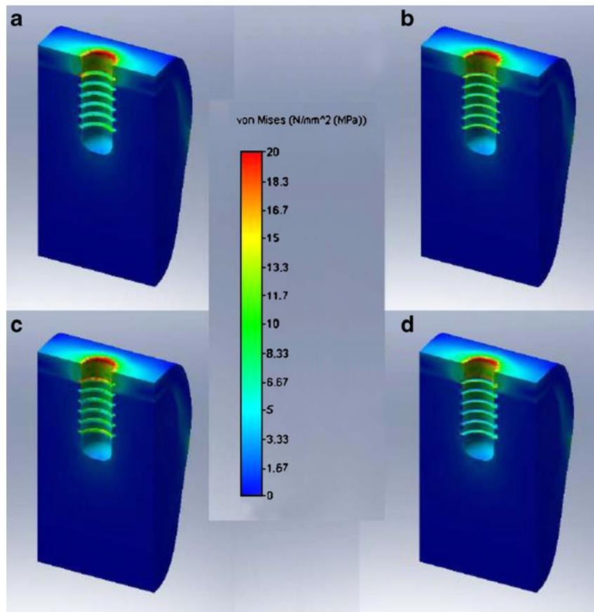
**Fig. 6** Distribution of compressive stresses (MPa) at mesiodistal cross-section, zoomed view of bone structure adjacent to cervical implant region. V-thread (a), buttress (b), reverse buttress (c), and square shape (d) threads. Blue to red colors represents stress values from lower to higher, respectively
