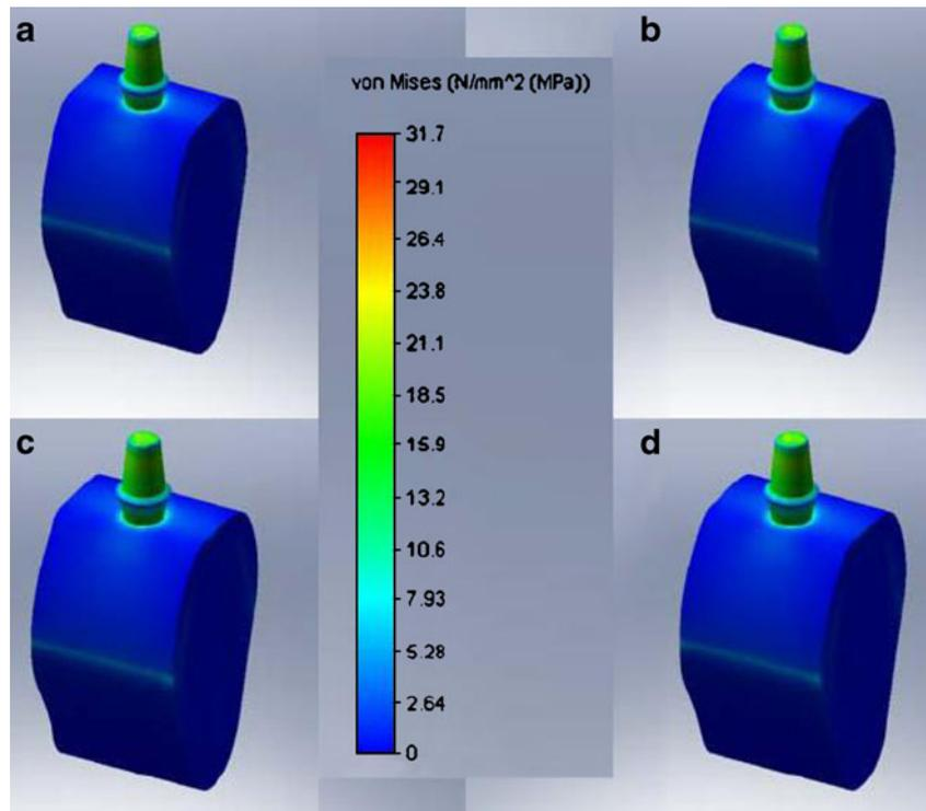
**Fig. 5** Distribution of von Mises stresses (MPa) at mesio-distal cross-section view of bone structure. V-thread (a), buttress (b), reverse buttress (c), and square shape (d) threads. Blue to red colors represents stress values from lower to higher, respectively
