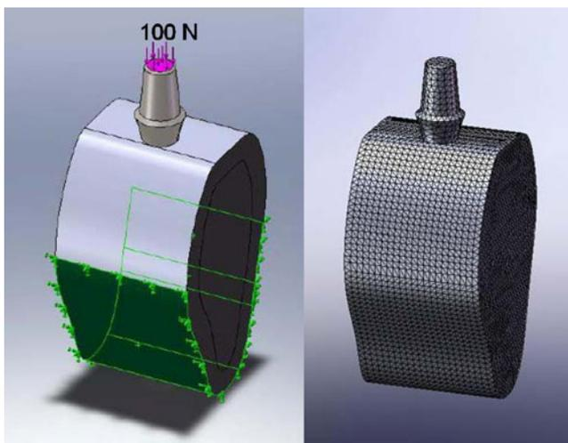
**Fig. 3** Illustration of 3D FE model, load application, and boundary condition. Pink arrow represents the load application, and green area is assumed as fixed as boundary condition
