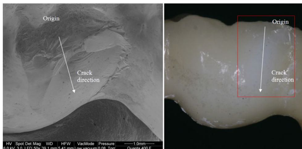
Fig. 2 Group 2: picture of the chipping area and SEM image (magnification)
