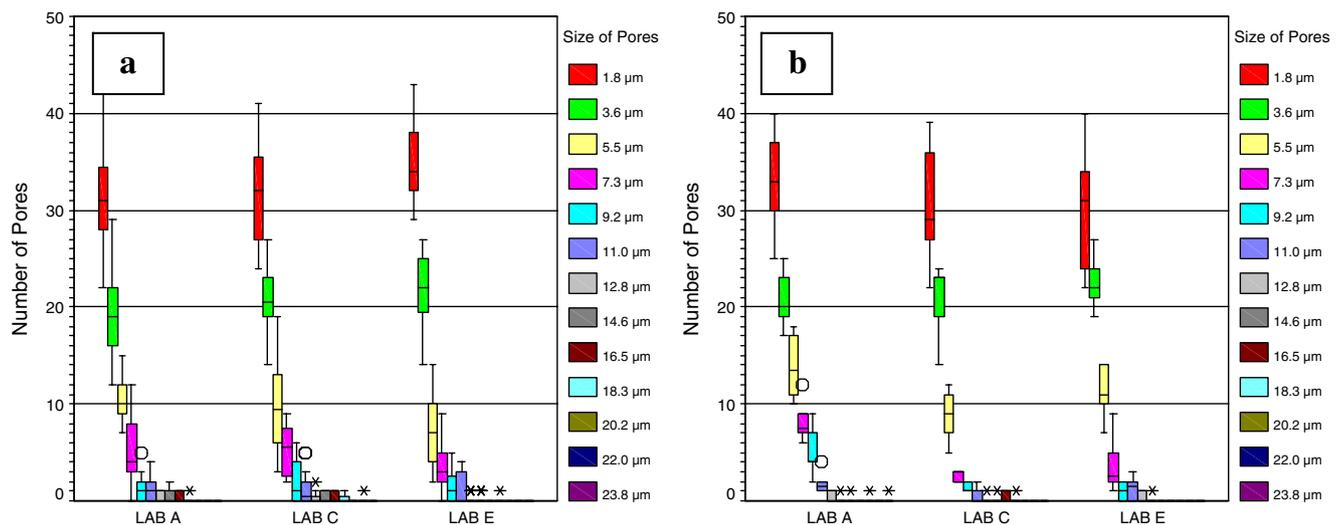
**Fig. 7** Comparison of the quantity of the shrinkage cavities made of AuPtZn alloy **a** for crowns and **b** for FDP pontics from different dental laboratories
