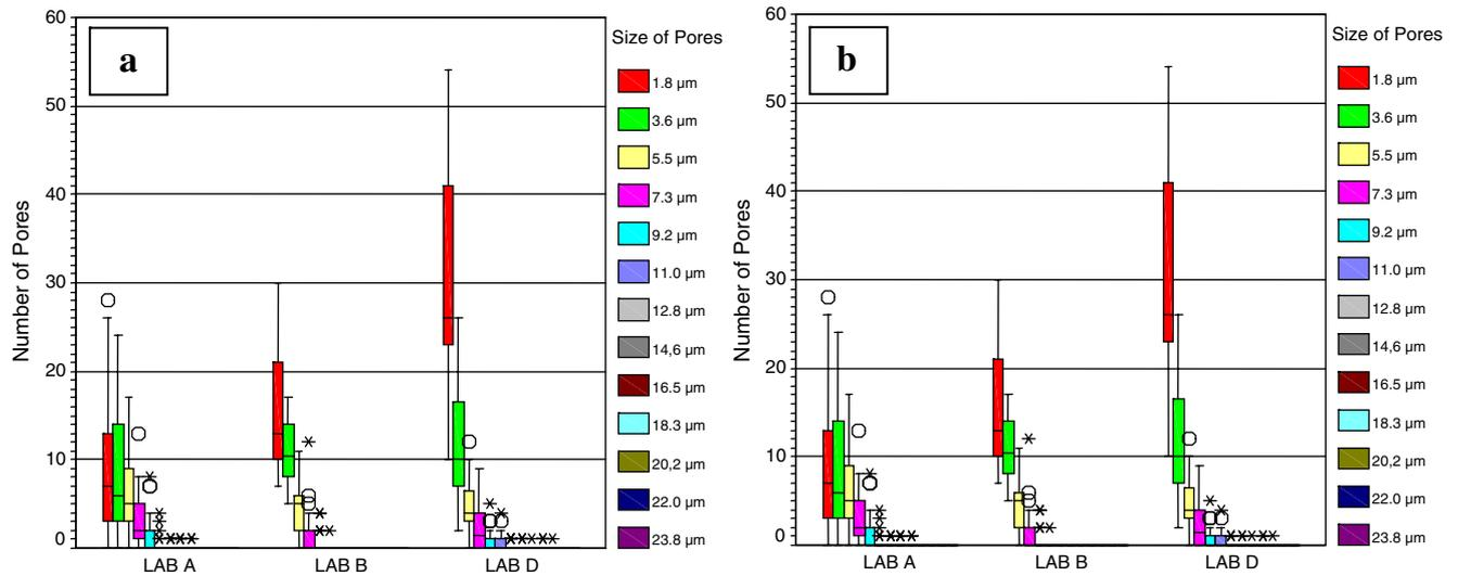
**Fig. 6** Comparison of the quantity of the shrinkage cavities made of AuAgCuPt alloy **a** for crowns and **b** for FDP pontics from different dental laboratories
