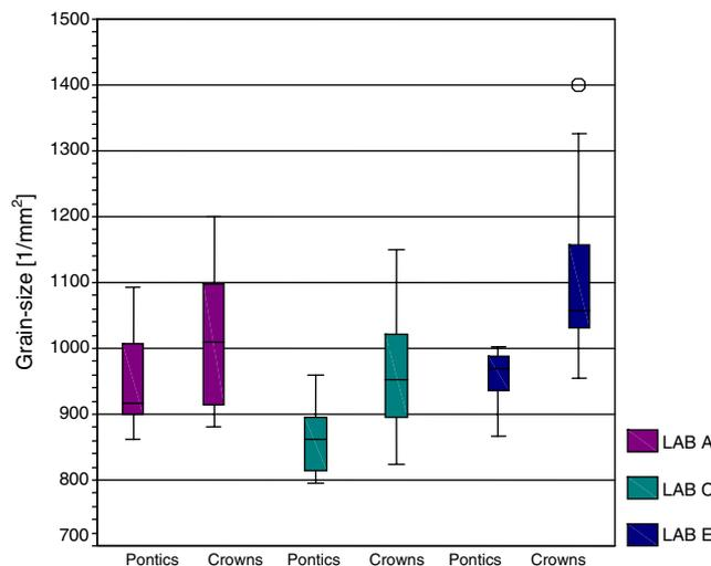
**Fig. 4** Comparison of the grain size [1/mm<sup>2</sup>] of crowns and pontics from different dental laboratories for the alloy AuPtZn alloy
