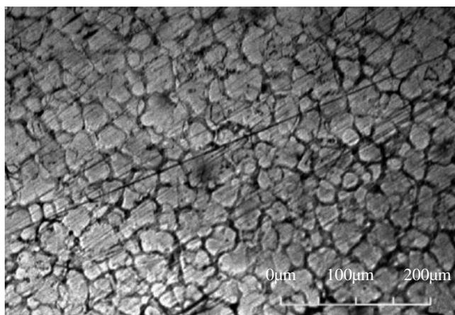
**Fig. 1** Microstructure of an AuAgCuPt alloy crown from Lab A with a grain size of 1,334/mm<sup>2</sup>
