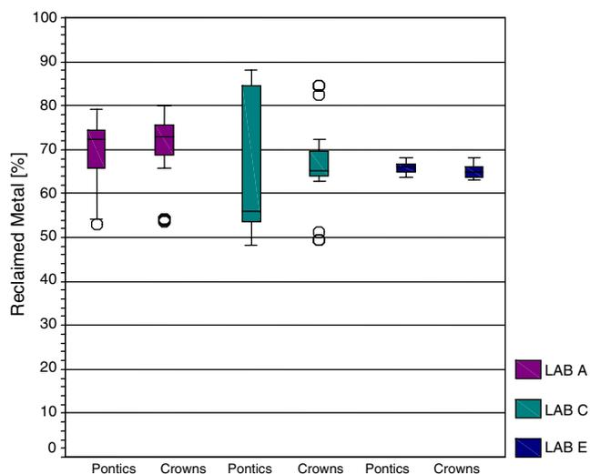
**Fig. 5** Comparison of the reclaimed metal of crowns and pontics from different dental laboratories for the AuPtZn alloy
