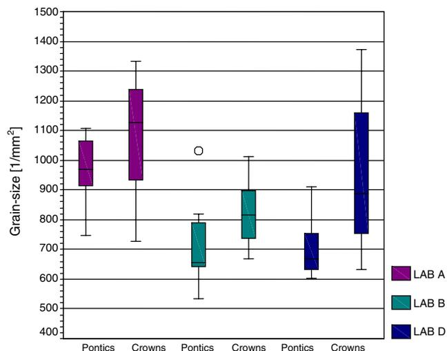
**Fig. 2** Comparison of the grain size [1/mm<sup>2</sup>] of crowns and pontics from different dental laboratories for the AuAgCuPt alloy
