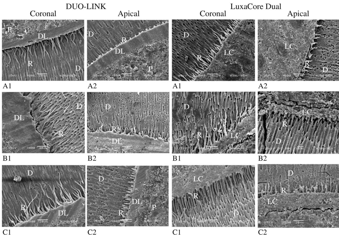
**Fig. 4** SEM examples of the interfaces between the dentine and the bonded DUO-LINK and LuxaCore Dual cements in the coronal and apical post space segments (the resin tag appearances in the middle post space segments were intermediate between those of the two other segments). *D* dentine, *R* resin tags, *P* D.T. LIGHT-POST, *DL* DUO-LINK cement, *LC* LuxaCore Dual cement. *A1, A2* Group A—0.9% NaCl 60 s: Sparse irregular resin tags lacking lateral branches were
