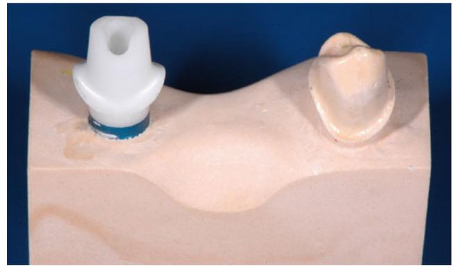
**Fig. 2** Master cast for test groups with implant–tooth supported restorations prepared for the scanning process
