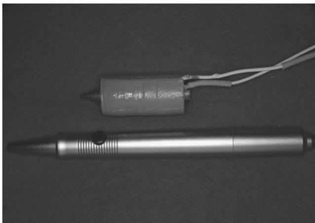
**Fig. 9** Ferrite rod wound with enamel wire of electromagnetic vibration device and hand-piece of Periotest®
