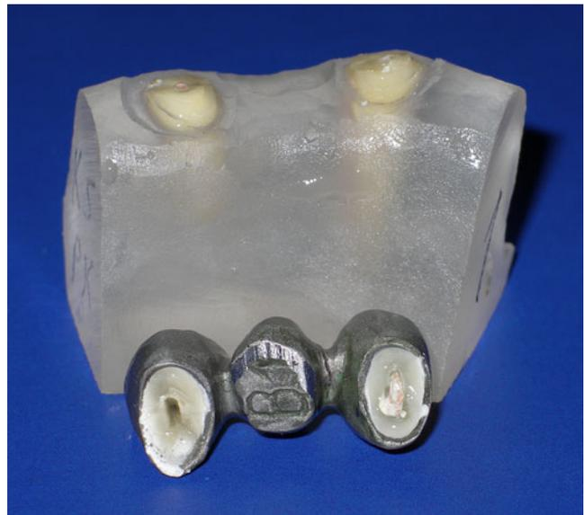
**Fig. 2** Example of type 3 failure pattern showing horizontal cervical root fracture of both the canine and the premolar teeth
