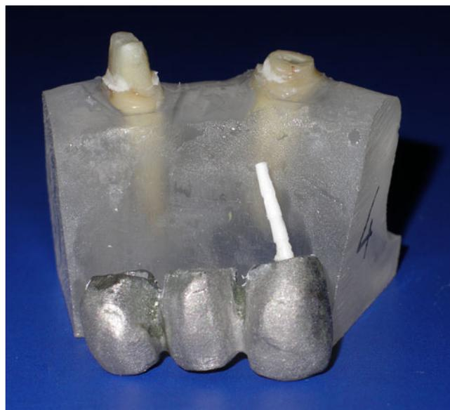
**Fig. 4** Typical root fractures in group 5 showing type 3 failure. Note the post core complex debonded
