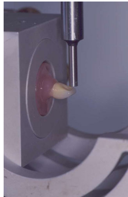
Fig. 2 Method of holding and loading test specimens
