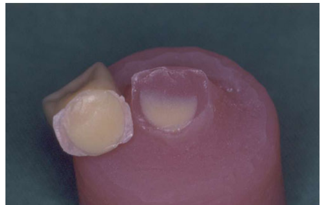
Fig. 4 Mixed adhesive/cohesive failure mode
