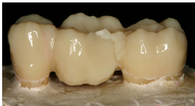
Fig. 2 Ceramic bulk fracture at the distal connector of a M-LiCAD FDP
