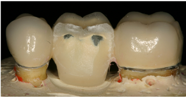
Fig. 4 Cohesive fracture within the veneering ceramic of a MC FDP exposing the metal core
