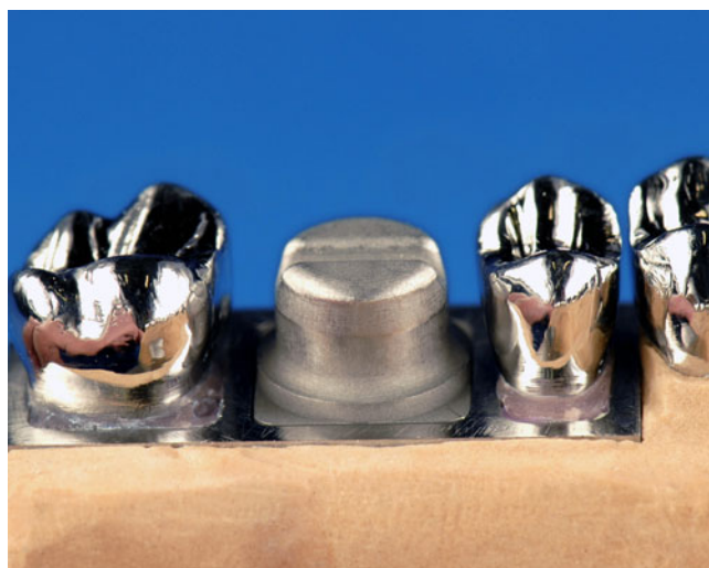
Fig. 2 A simplified tooth model with a circular chamfer preparation, a circular parallel area, and a conical area on top
