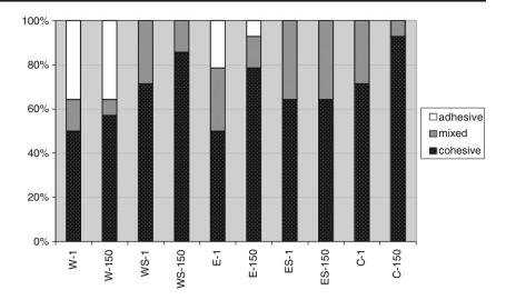
Cleaning the silanized glass ceramic surface with only a water spray resulted in significantly lower bond strength to the leucite-reinforced glass ceramic compared to the uncontaminated control group after long-term storage in Ringer's solution. It was not possible to achieve a durable long-term bond with this procedure. Therefore, the null hypothesis was disproved.
