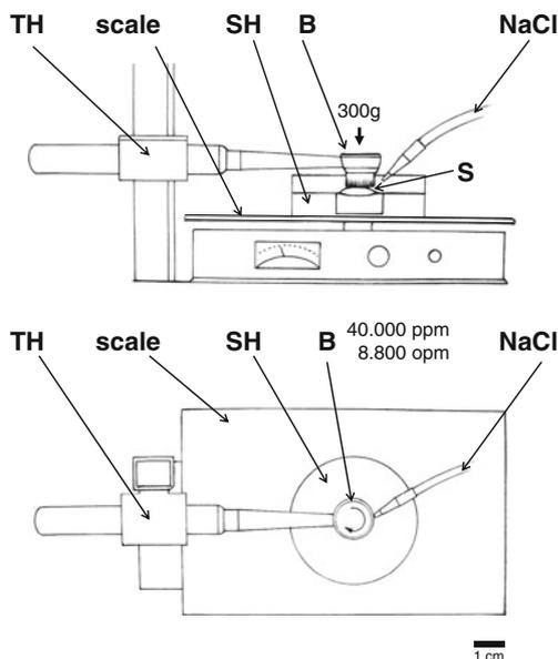
**Fig. 1** A schematic diagram of the toothbrush abrasion testing device: Each specimen (S) was fixed on a specimen holder (SH). A power toothbrush (B) conducting 40,000 pulsations/min and 8,800 oscillations/min was fixed in a toothbrush holder (TH) and was set to give the specimen (S) 300 g vertical load (controlled by a scale). Scale bar indicates 1 cm
