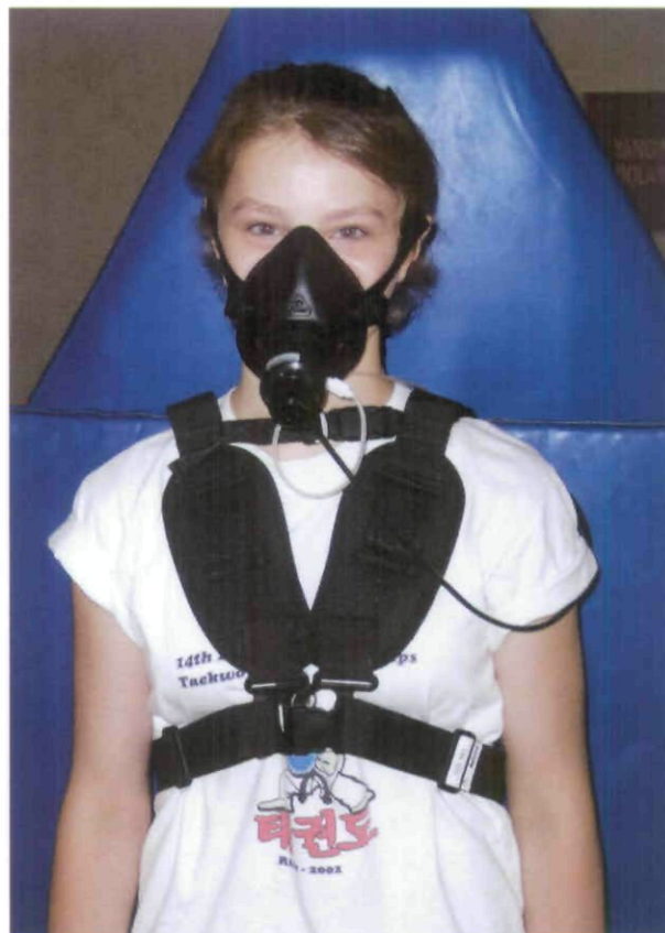
Fig. 4. Breath-by-breath data collected through a face mask and sent to a host computer system via wireless transmission (telemetry).
