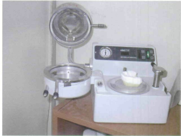
Fig. 1. Thermal forming machine used for the fabrication of mouth guards.
