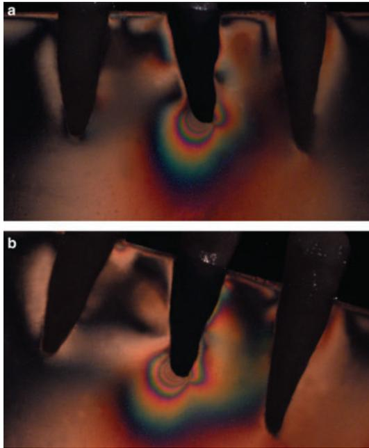
Fig. 1. (a, b) Isochromatic fringe orders around non-splinted tooth under static axial and 20° oblique force of 100 N. Note that stresses around the cervical and apical parts are compressive in nature under axial loading, whereas a combination of tensile and compressive stresses are generated under oblique load.
