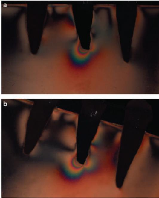
Fig. 3. (a, b) Isochromatic fringe orders around traumatized tooth splinted with orthodontic wire under static axial and 20° oblique force of 100 N.
