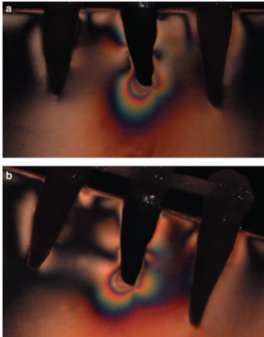
Fig. 4. (a, b) Isochromatic fringe orders around traumatized tooth splinted with ribbon under static axial and 20° oblique force of 100 N. Note the similarity in generation of isochromatic fringe orders around the tooth splinted by ribbon and titanium trauma splint under oblique load.
