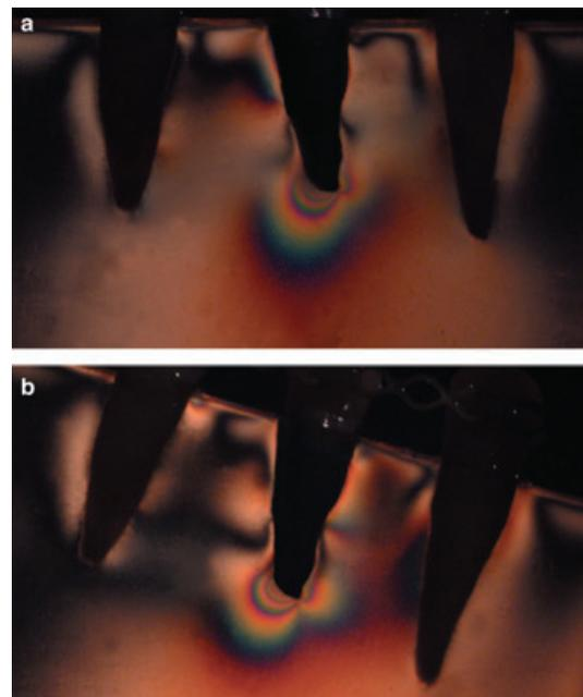
Fig. 2. (a, b) Isochromatic fringe orders around splinted tooth with titanium trauma splint under static axial and 20° oblique force of 100 N.
