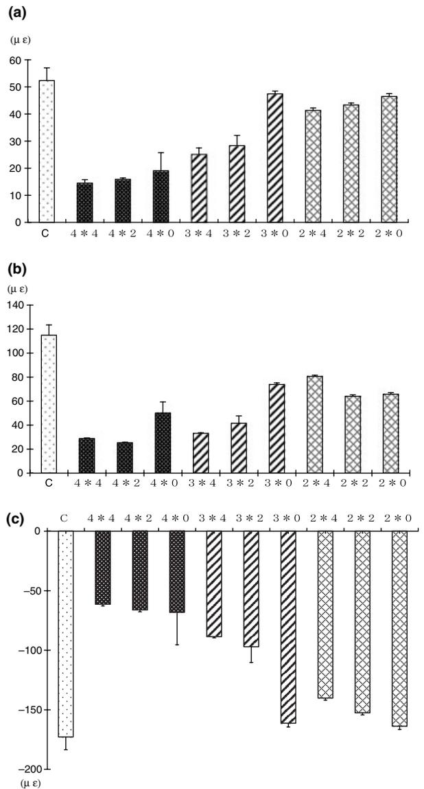
Fig. 6. (a–c) Outputs from three strain gauges with the calibrated shock delivered from the front (the thickness of the sheet \* the palatal margin location). (a) Strains at the labial-cervical surface, (b) strains at the palatal-root surface, and (c) strains on the palatal-alveolar bone surface.
