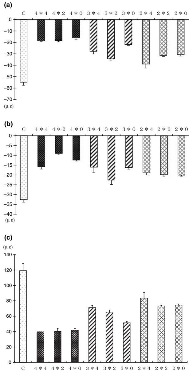
Fig. 7. (a–c) Outputs from three strain gauges with the calibrated shock delivered in the upper anterior direction (the thickness of the sheet \* the palatal margin location). (a) Strains at the labial-cervical surface, (b) strains at the palatal-root surface, and (c) strains on the palatal-alveolar bone surface.
