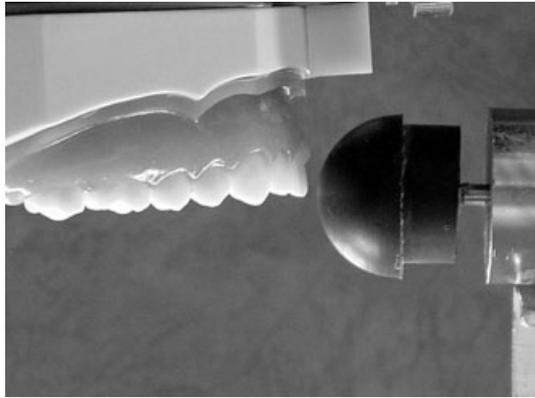
Fig. 1. Picture of a maxillary phantom model with maxillary teeth, bone, and soft tissue.
