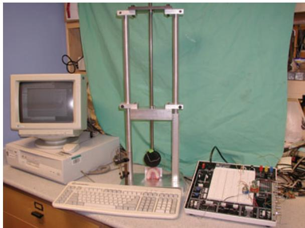
Fig. 3. The impact device and custom amplifier.
