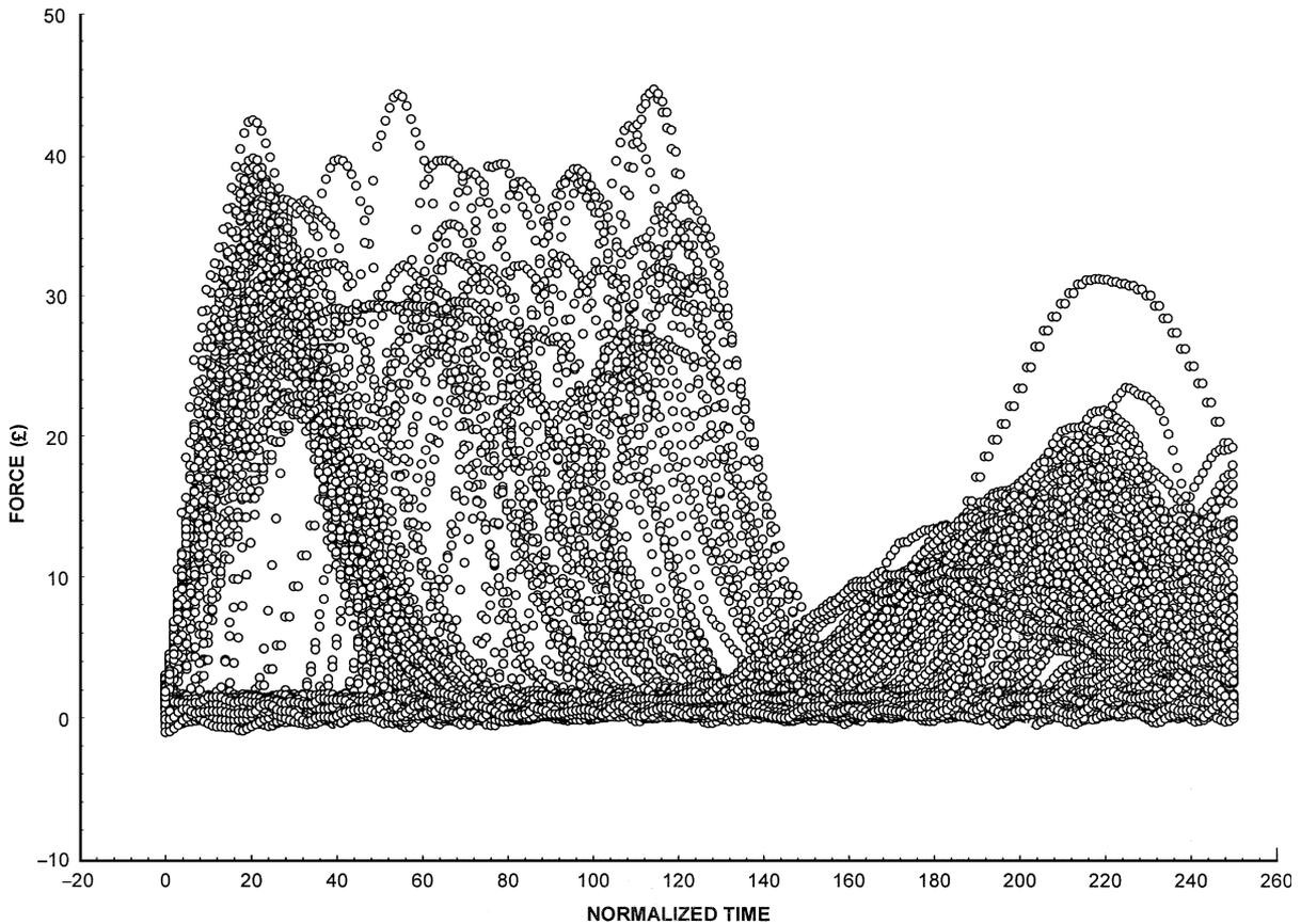
Fig. 2. Raw data – recorded force by location for 9mm drop height.
