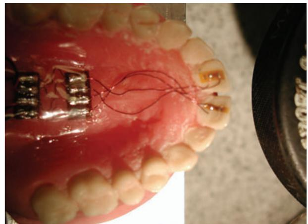
Fig. 4. Strain gauges in place.
