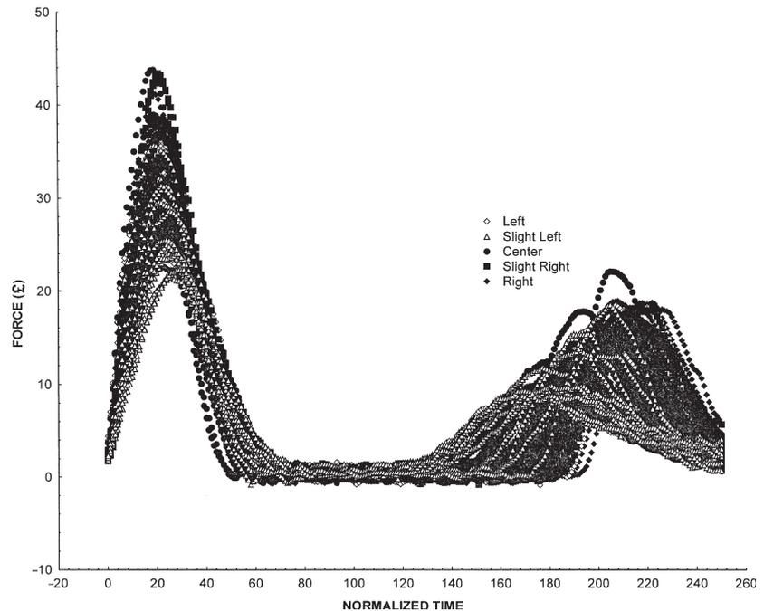
Fig. 5. Force by location for 9mm drop height.
