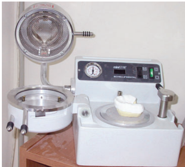
Fig. 1. Mouthguards were fabricated using a thermal-forming machine (MiniSTAR, Scheu-Dental, USA).
