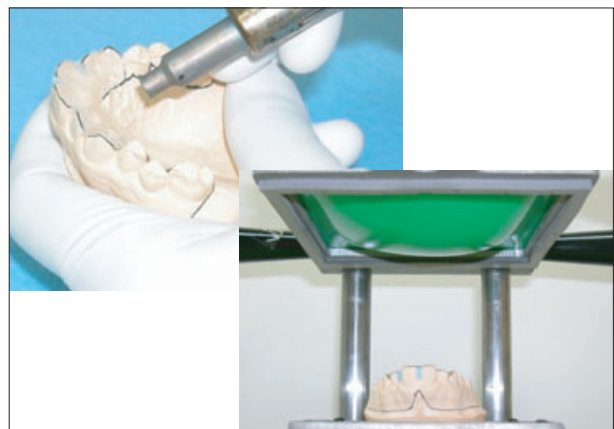
Fig. 6. Vacuum moulding of the second EVA material layer.
